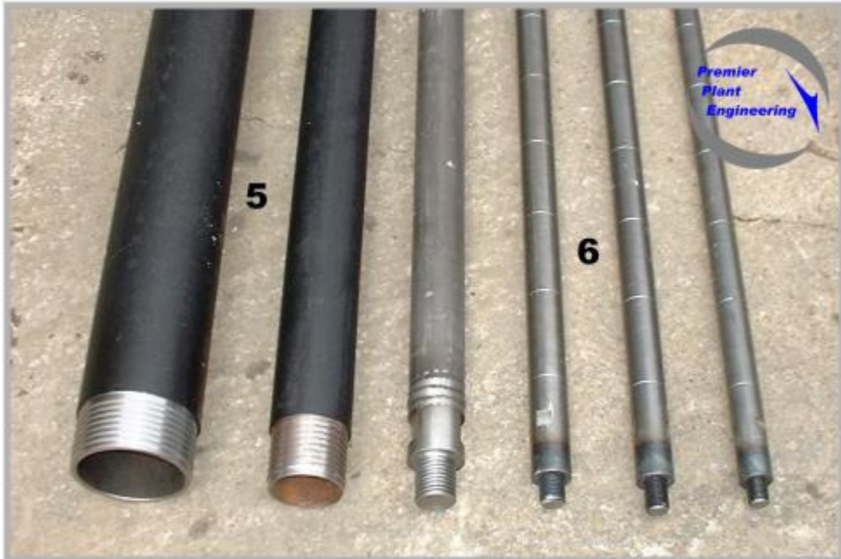
Above is a range of samplers, casing and rods that are used in the drill operation 1. SPT sampler 2. Window sampler 3. Windowless sampler 4. U 100 sampler 5. Casing 6. Various drill rods
