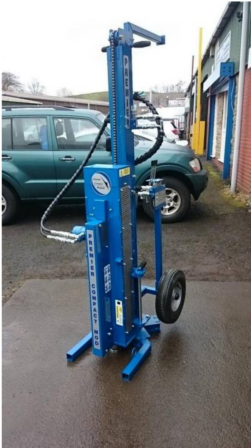
Figure 4 Showing the rig in the wheeled transport position (630mm wide). In this setup the rig can stand vertical as in the picture or laid down resting on its travel rest ideal for transportation in a vehicle.
